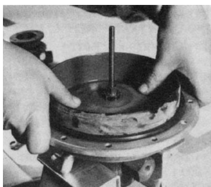
Figure 4-10 Removing cylinder from lower housing.
