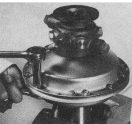
Figure 4-6 Removing housing screws and nuts.
