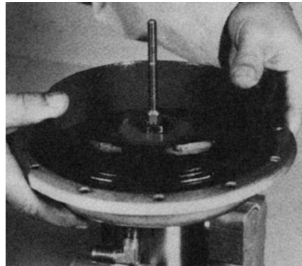
Figure 7-7 Pressing cylinder into lower housing.
