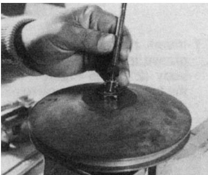
Figure 7-3 Connecting rod with lock washer and shifting nut, ready to be screwed into fluid piston.
