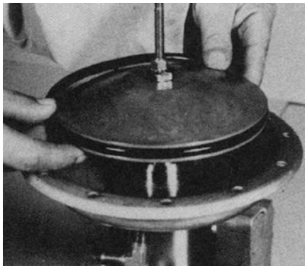
Figure 7-6 Inserting air piston and fluid piston assembly into fluid body.
