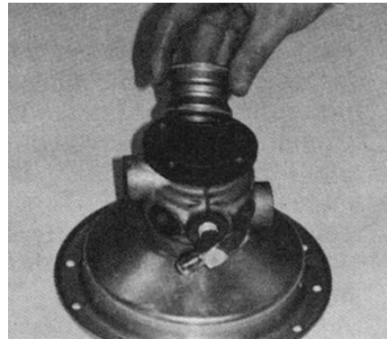
Figure 7-8 Inserting J type shuttle assembly into air valve body.
