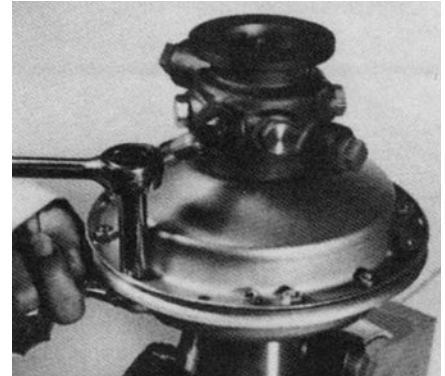
Figure 7-10 Bolting upper and lower housings together.
