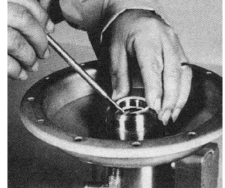
Figure 7-5 Installing seals in fluid body.
