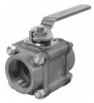
Category: Worcester 44 [1] row: 484 Product series: 44 Body pipe ends: CARBON STEEL Ball and stem: BRASS Seats and seals: HIGH-PER FILL SEATS G SEALS End connections: SCREWED ENDS FNPT Brand: Worcester [2] Series: series 44 [3] Item series: series 44 [4]
