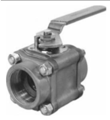
Category: Worcester 44 [1] row: 899 Product series: 44 Body pipe ends: STAINLESS STEEL Ball and stem: BRASS Seats and seals: TEFLON SEATS EPR SEALS End connections: SOCKET WELD Brand: Worcester [2] Series: series 44 [3] Item series: series 44 [4]
