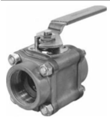
Category: Worcester 44 [1] row: 1683 Product series: 44 Body pipe ends: CARBON STEEL Ball and stem: BRASS Seats and seals: HIGH-PER FILL SEATS G SEALS End connections: SOCKET WELD Brand: Worcester [2] Series: series 44 [3] Item series: series 44 [4]
