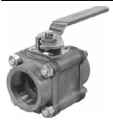
Category: Worcester 44 [1] row: 1830 Product series: 44 Body pipe ends: CARBON STEEL Ball and stem: STAINLESS STEEL Seats and seals: TEFLON SEATS EPR SEALS End connections: SOCKET WELD Brand: Worcester [2] Series: series 44 [3] Item series: series 44 [4]
