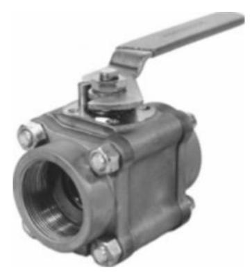
Category: Worcester 44 [1] row: 3174 Product series: 44 Body pipe ends: CARBON STEEL Ball and stem: MONEL Seats and seals: POLYFILL SEATS VITON SEALS End connections: SOCKET WELD Brand: Worcester [2] Series: series 44 [3] Item series: series 44 [4]
