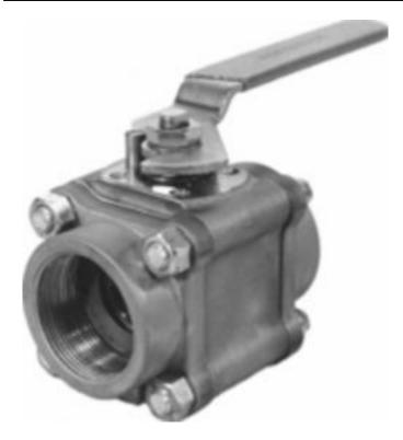
Category: Worcester 44 [1] row: 4147 Product series: 44 Body pipe ends: CARBON STEEL Ball and stem: STAINLESS STEEL Seats and seals: REINFORCED TEFLON SEATS TEFLON SEALS End connections: SOCKET WELD Brand: Worcester [2] Series: series 44 [3] Item series: series 44 [4]
