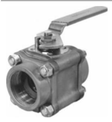
Category: Worcester 44 [1] row: 4187 Product series: 44 Body pipe ends: CARBON STEEL Ball and stem: STAINLESS STEEL Seats and seals: REINFORCED TEFLON SEATS VITON SEALS End connections: SCREWED ENDS FNPT Brand: Worcester [2] Series: series 44 [3] Item series: series 44 [4]
