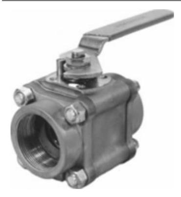
Category: Worcester 44 [1] row: 5650 Product series: 44 Body pipe ends: STAINLESS STEEL Ball and stem: BRASS Seats and seals: REINFORCED TEFLON SEATS VITON SEALS End connections: SCREWED ENDS FNPT Brand: Worcester [2] Series: series 44 [3] Item series: series 44 [4]
