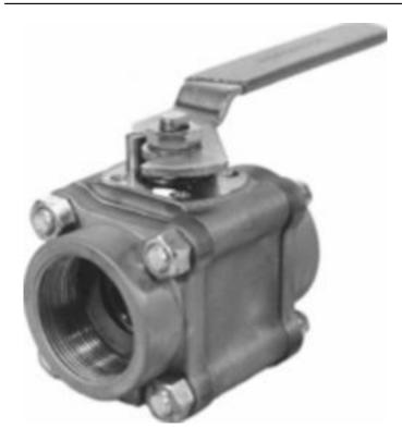
Category: Worcester 44 [1] row: 5922 Product series: 44 Body pipe ends: STAINLESS STEEL Ball and stem: MONEL Seats and seals: REINFORCED TEFLON SEATS VITON SEALS End connections: EXTENDED BUTT WELD Brand: Worcester [2] Series: series 44 [3] Item series: series 44 [4]
