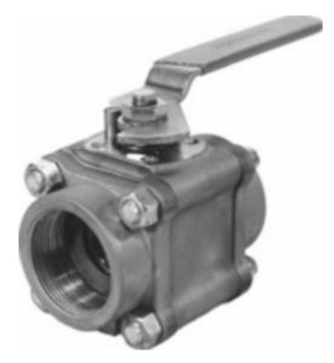
Category: Worcester 44 [1] row: 6441 Product series: 44 Body pipe ends: CARBON STEEL Ball and stem: BRASS Seats and seals: TEFLON SEATS VITON SEALS End connections: SCREWED ENDS FNPT Brand: Worcester [2] Series: series 44 [3] Item series: series 44 [4]
