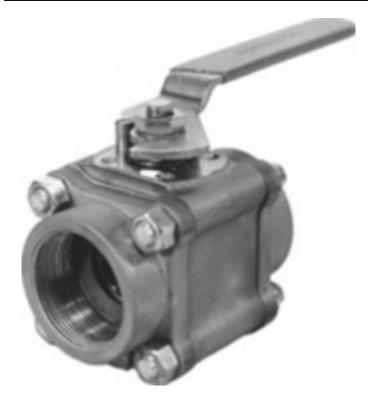
Category: Worcester 44 [1] row: 7654 Product series: 44 Body pipe ends: CARBON STEEL Ball and stem: BRASS Seats and seals: LUBETAL SEATS VITON SEALS End connections: SOCKET WELD Brand: Worcester [2] Series: series 44 [3] Item series: series 44 [4]
