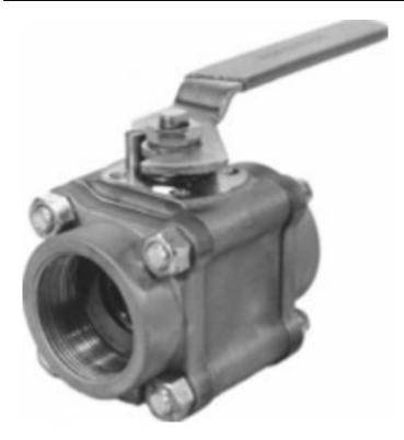
Category: Worcester 44 [1] row: 7738 Product series: 44 Body pipe ends: CARBON STEEL Ball and stem: STAINLESS STEEL Seats and seals: REINFORCED TEFLON SEATS TEFLON SEALS End connections: SOCKET WELD Brand: Worcester [2] Series: series 44 [3] Item series: series 44 [4]
