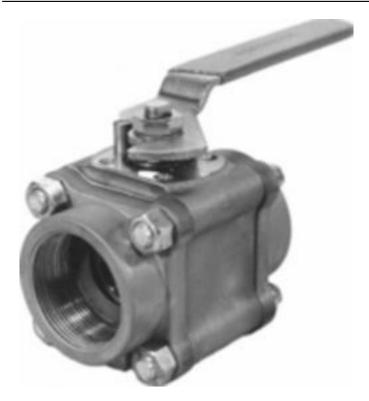
Category: Worcester 44 [1] row: 8711 Product series: 44 Body pipe ends: BRASS Ball and stem: MONEL Seats and seals: REINFORCED TEFLON SEATS VITON SEALS End connections: SOCKET WELD Brand: Worcester [2] Series: series 44 [3] Item series: series 44 [4]
