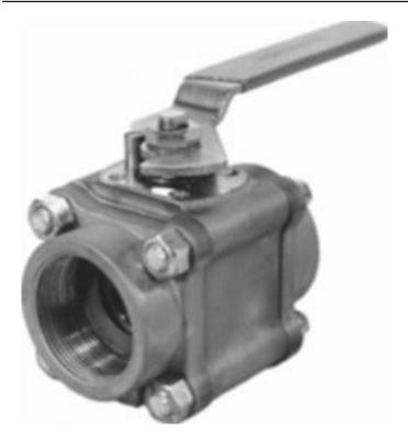
Category: Worcester 44 [1] row: 173 Product series: 44 Body pipe ends: BRASS Ball and stem: MONEL Seats and seals: REINFORCED TEFLON SEAT VITON SEAL End connections: SCREWED ENDS FNPT Brand: Worcester [2] Series: series 44 [3] Item series: series 44 [4]
