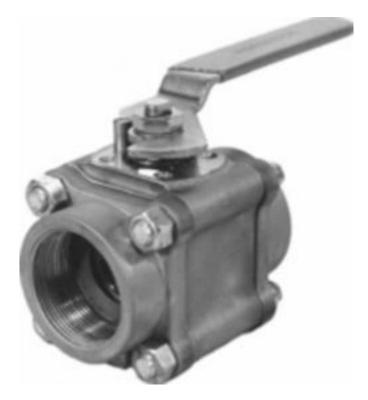
Category: Worcester 44 [1] row: 406 Product series: 44 Body pipe ends: CARBON STEEL Ball and stem: MONEL Seats and seals: POLYFILL SEAT VITON SEAL End connections: BUTT WELD Brand: Worcester [2] Series: series 44 [3] Item series: series 44 [4]
