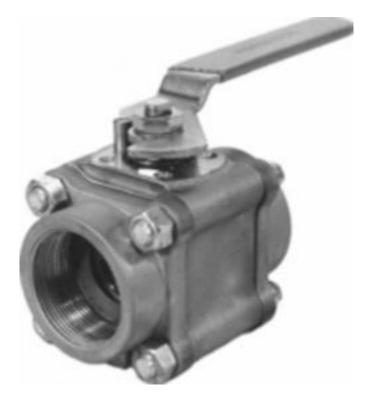
Category: Worcester 44 [1] row: 382 Product series: 44 Body pipe ends: CARBON STEEL Ball and stem: MONEL Seats and seals: LUBETAL SEAT VITON SEAL End connections: BUTT WELD Brand: Worcester [2] Series: series 44 [3] Item series: series 44 [4]
