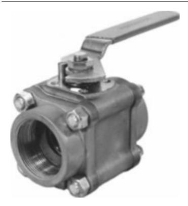
Category: Worcester 44 [1] row: 446 Product series: 44 Body pipe ends: STAINLESS STEEL Ball and stem: BRASS Seats and seals: REINFORCED TEFLON SEAT VITON SEAL End connections: BUTT WELD Brand: Worcester [2] Series: series 44 [3] Item series: series 44 [4]
