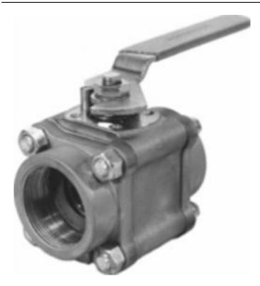
Category: Worcester 44 [1] row: 597 Product series: 44 Body pipe ends: STAINLESS STEEL Ball and stem: MONEL Seats and seals: TEFLON SEAT M SEAL End connections: SCREWED ENDS FNPT Brand: Worcester [2] Series: series 44 [3] Item series: series 44 [4]
