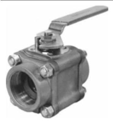
Category: Worcester 44 [1] row: 553 Product series: 44 Body pipe ends: STAINLESS STEEL Ball and stem: MONEL Seats and seals: TEFLON SEAT AND SEAL End connections: SCREWED ENDS FNPT Brand: Worcester [2] Series: series 44 [3] Item series: series 44 [4]
