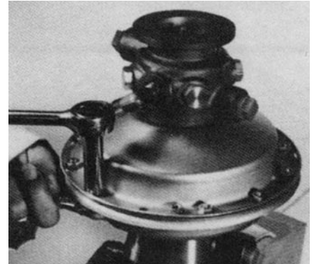
Figure 7-10 Bolting upper and lower housings together.
