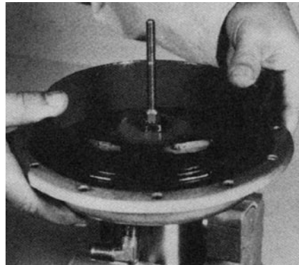
Figure 7-7 Pressing cylinder into lower housing.
