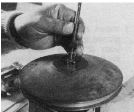
Figure 7-3 Connecting rod with lock washer and shifting nut, ready to be screwed into fluid piston.
