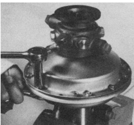
Figure 4-6 Removing housing screws and nuts.
