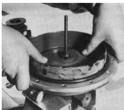
Figure 4-10 Removing cylinder from lower housing.
